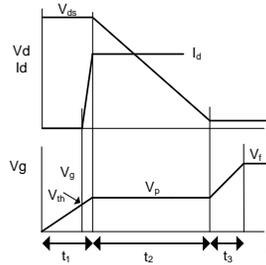
Figure 2. Turn-on Characteristics
