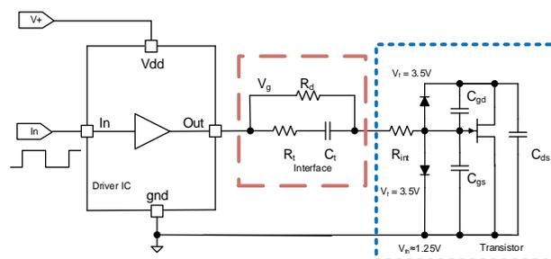
**Figure 1. Interface for NexGen's e-mode Vertical GaN™ JFET. The blue short dashed box shows the JFET model and the large dashed red box shows the interface model. The standard driver is on the left.**
