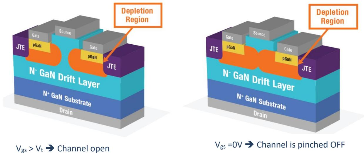
Figure 3: Conceptual view of Vertical GaN™ channel control principle
