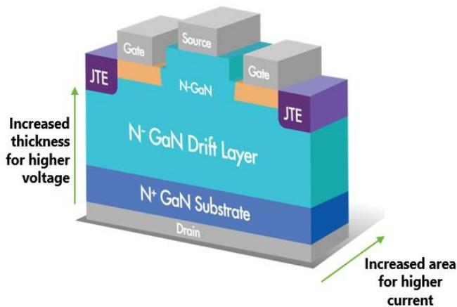
Figure 2 : Vertical GaN™ cross-section, conceptual view
