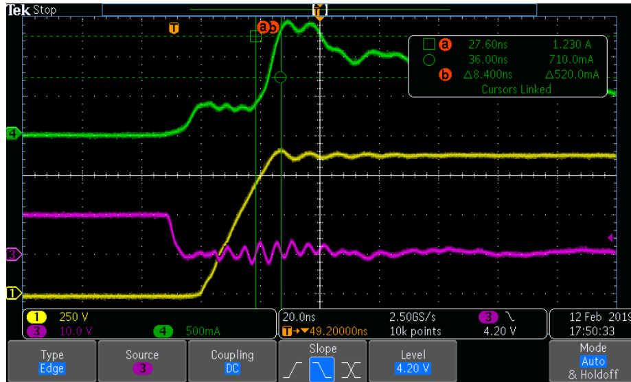
Figure 10: Transistor turn off with Diode Current 20nsec/div, Yellow Vds 250V/div, Purple Cascode MOSFET gate drive 10V/div, Green Boost Diode Current 500mA/div.
