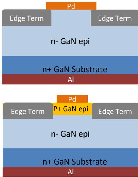
Figure 1. Schematic cross-sections of SBDs and PN diodes
