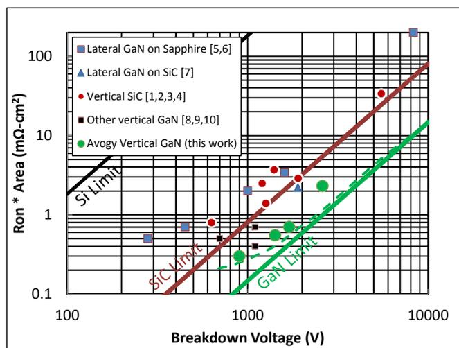
Figure 5. Power device FOM plot comparing Avogy vertical GaN diodes with other SiC, lateral GaN, and vertical GaN devices
