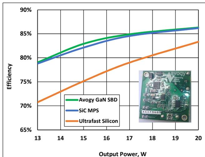
Figure 6. Efficiency comparison of vertical GaN, SiC, and Si diodes in an off-line LED driver circuit
