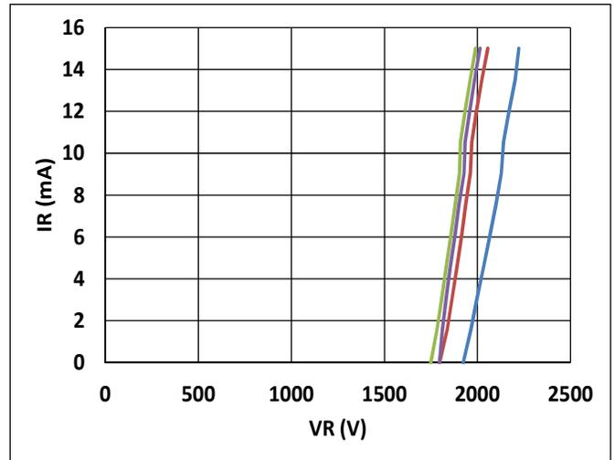
Figure 4. Pulsed reverse I-V characteristics of PN Diodes
