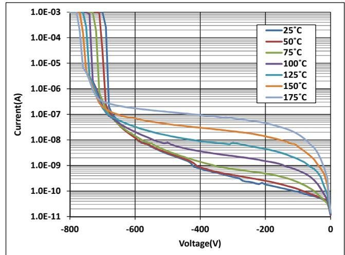
Figure 3. Reverse I-V characteristics of PN diodes as a function of temperature.
