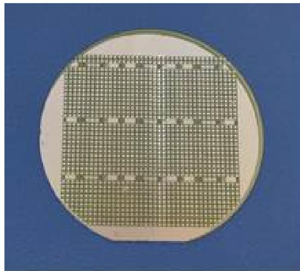
Figure 7. A 2-inch bulk GaN wafer with fabricated diodes
