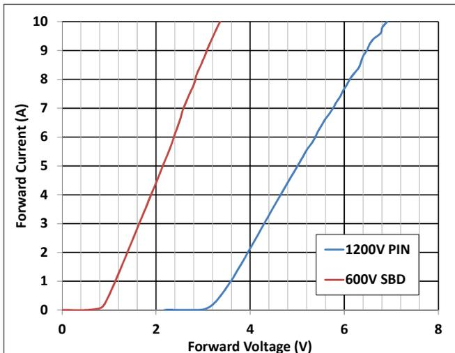
Figure 2. Pulsed forward I-V characteristics of SBDs and PN diodes
