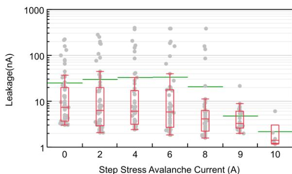
Figure 5b) Statistics of reverse current at a reverse bias of 600 V for devices surviving after each repetitive avalanche stress step. “0A” indicates incoming population. The plot shows the reverse current for individual devices with dots, the box-plot and the mean line.
