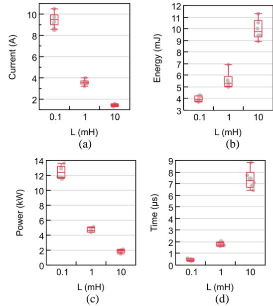
Figure 3) Distribution of various pulse parameters for the smallest current pulse that results in device destruction: a) peak inductive avalanche current, b) Energy deposited into the device, c) Peak power dissipated on the device, and d) Time to onset of breakdown
