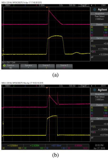
Figure 2: Scope waveforms displaying DUT current (purple) and the voltage (yellow): a) normal avalanche, and b) destructive avalanche
