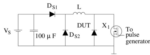
Figure 1) Avalanche test circuit. D<sub>S1</sub> and D<sub>S2</sub> are Schottky diodes, X<sub>1</sub> is the switch with the gate controlled by an external pulse generator. L is the load inductor and the DUT is the device under test.
