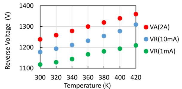
Figure 4: Breakdown voltage ( $V_R$ ) and avalanche voltage ( $V_A$ ) as a function of temperature. Breakdown voltage  $V_R$  is the reverse voltage measured using an SMU under 1mA and 10mA reverse current. The avalanche voltage is measured under 2 A peak inductive pulse supplied from a 1mH inductor.
