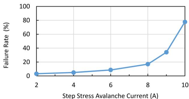
Figure 5a) Incremental failure rate at each test step
