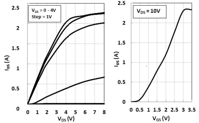
Fig. 3. DC output and transfer characteristics of the vertical GaN transistor.
