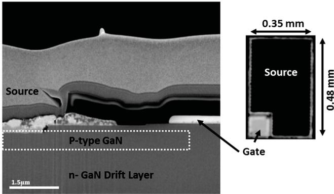
Fig. 2. Transistor cross section and top view image.
