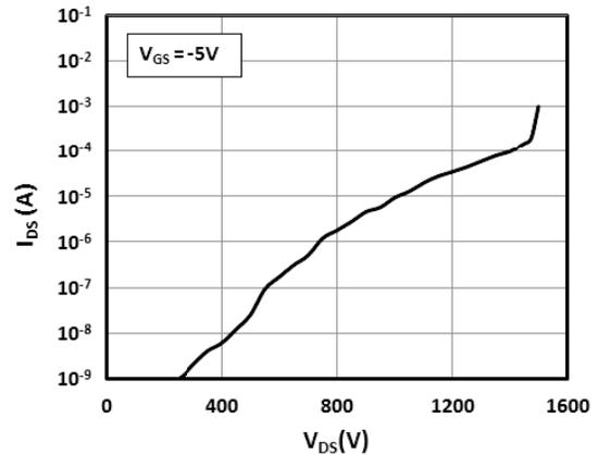
Fig. 4. Reverse current-voltage characteristics of the vertical GaN transistor.
