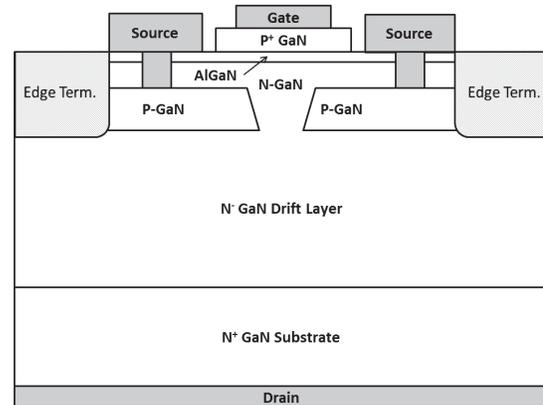
Fig. 1. Schematic cross-section the vertical GaN transistor on bulk GaN.
