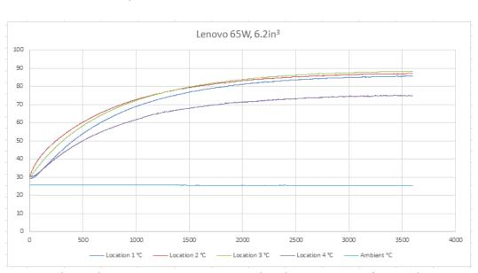
The picture above shows temperature measured at the outer case of a 65W laptop power adapter. After one hour, the hot spots on the case have risen to just under 90C or 193F! This adapter carries the brand of a well known OEM, and carries the UL safety mark.
