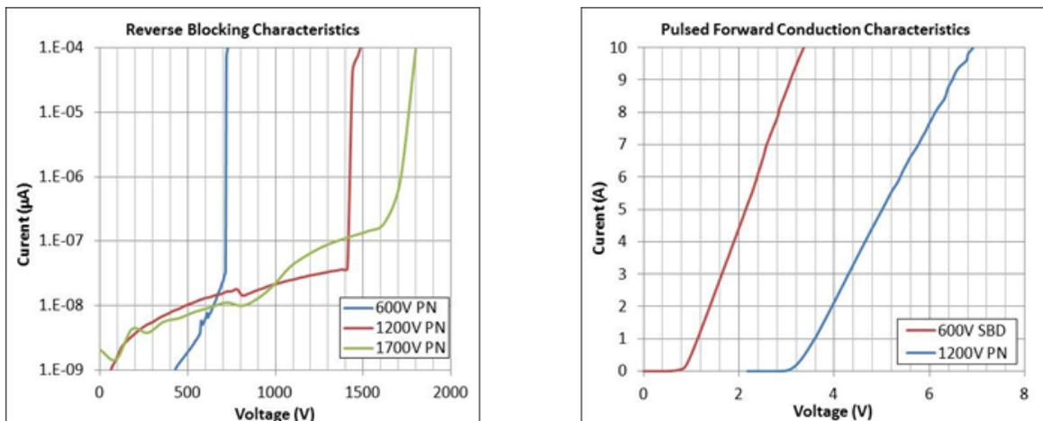
Fig. 2. Measured I-V characteristics of GaN-on-GaN Schottky barrier diodes and pn diodes.
