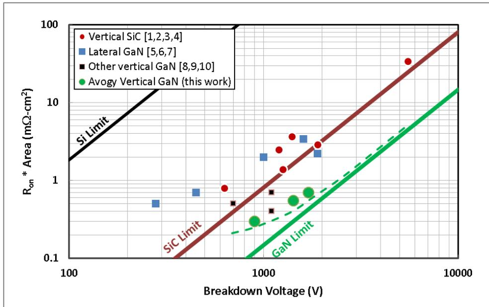
Fig. 3. Theoretical and reported specific on-resistance ( $R_{sp}$ ) vs. breakdown voltage (BV).
