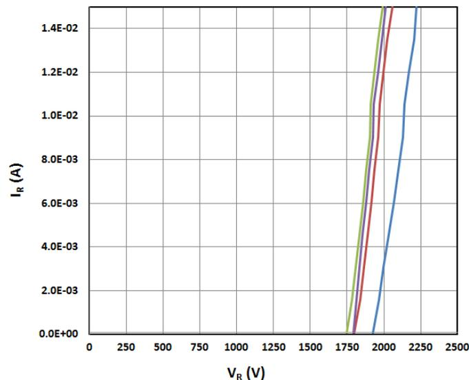
Fig. 4. GaN pn diodes with avalanche capability and >900 mJ of avalanche power.
