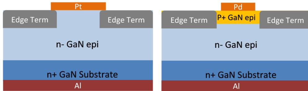
Fig. 1. Schematic cross sections of vertical GaN Schottky diode and pn diode.
